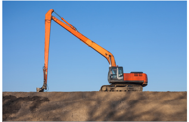
A long arm excavator will be used
